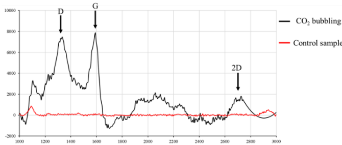
Figure 9. Raman spectroscopy from control and Mg-Gr composite.
